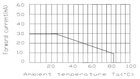
For operation above 25 °C,The lfm & Pd must be derated , the current derating is -0.36mA/ °C for DC drive and -0.86mA/ °C for Pulse drive ,the Power dissipation is -0.75mW/ °C.The product working current must not more than the 60% of the lfm or Ifp according to the working temperature.
