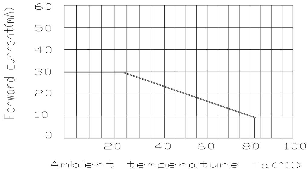
For operation above  $25\text{ }^{\circ}\text{C}$ , The  $I_{fm}$  &  $P_d$  must be derated, the current derating is  $-0.36\text{mA}/^{\circ}\text{C}$  for DC drive and  $-0.86\text{mA}/^{\circ}\text{C}$  for Pulse drive, the Power dissipation is  $-0.75\text{mW}/^{\circ}\text{C}$ . The product working current must not more than the 60% of the  $I_{fm}$  or  $I_{fp}$  according to the working temperature.
